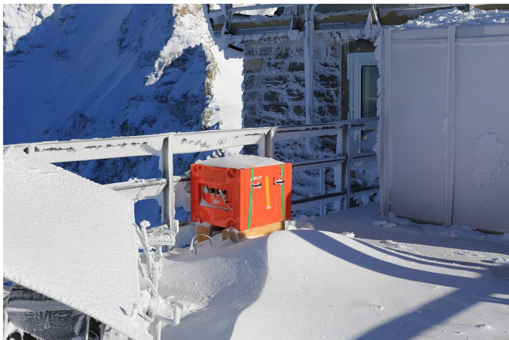
*Figure 1. Methanol Fuel Cell in its new weatherproof aluminium box on the lower platform of the Sphinx observatory during the winter trials.*
