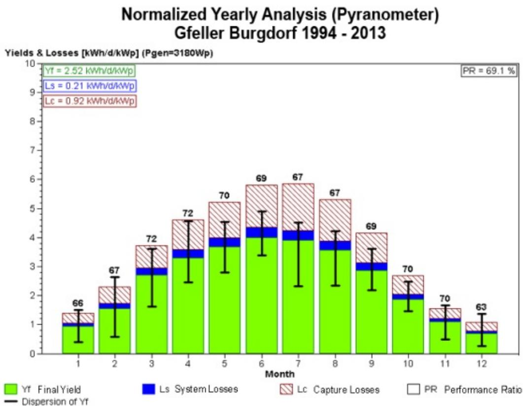
Figure 5. Typical energy production with a photovoltaic power plant in the Swiss basin (big earnings in the summer, low earnings in the winter).
