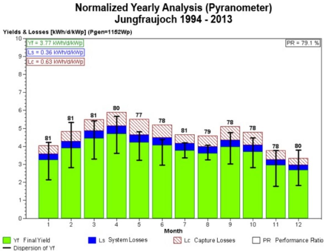
Figure 6. Distribution of energy produced with the photovoltaic power plant at Jungfraujoch evidencing a smaller seasonal variation than at PV installations in the Swiss basin (shown in Figure 5).
