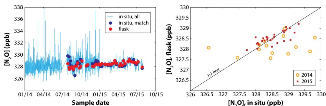
Figure 1. Comparison of N<sub>2</sub>O mole fractions measured in flask samples using QCLAS at the Empa GAW-WCC lab and in situ at Jungfraujoch using GC-ECD or OA-ICOS in 2014 and 2015, respectively (data courtesy of M. Steinbacher, Empa). The limited compatibility in 2014, was mainly due to the restricted performance of the in-situ analytical technique (GC-ECD).
