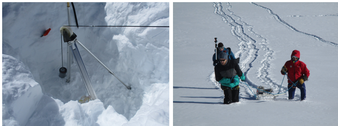
Figure 2. Field work activities at CG during the campaign of September 2016. Left: borehole inclination measurements. Right: GPR and surface topography measurements.
