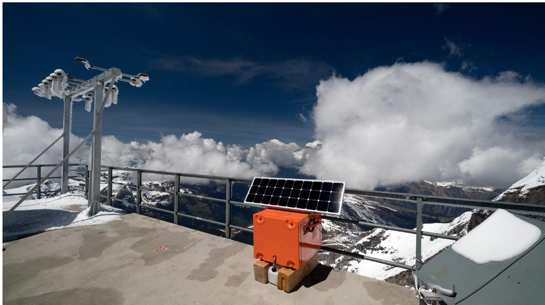
*Figure 1. Methanol Fuel Cell in its weatherproof aluminium box with the attached auxiliary solar panel on the lower platform of the Sphinx observatory during the May trials.*
