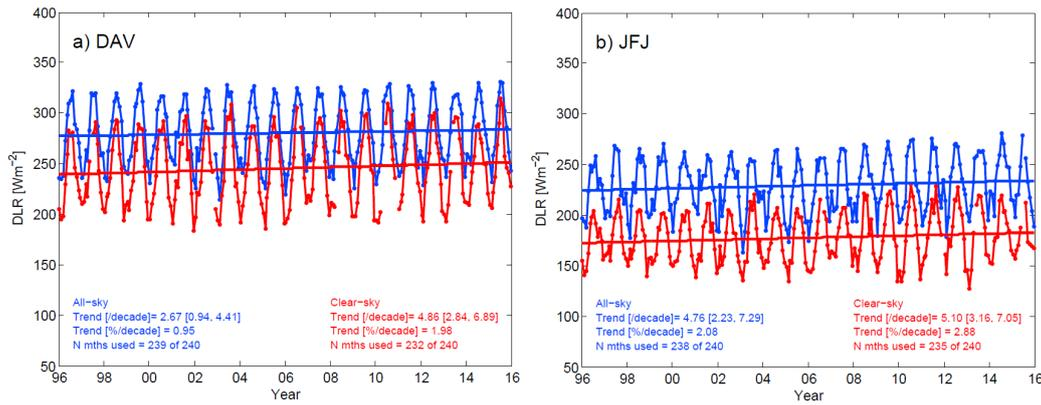
Figure 1. Monthly average DLR values during all-sky (blue) and clear-sky (red) conditions at: a) Davos and b) Jungfraujoch. Each panel also shows trend results from linear least squares analysis. Values in brackets represent the upper and lower bounds of the 90% confidence interval.
