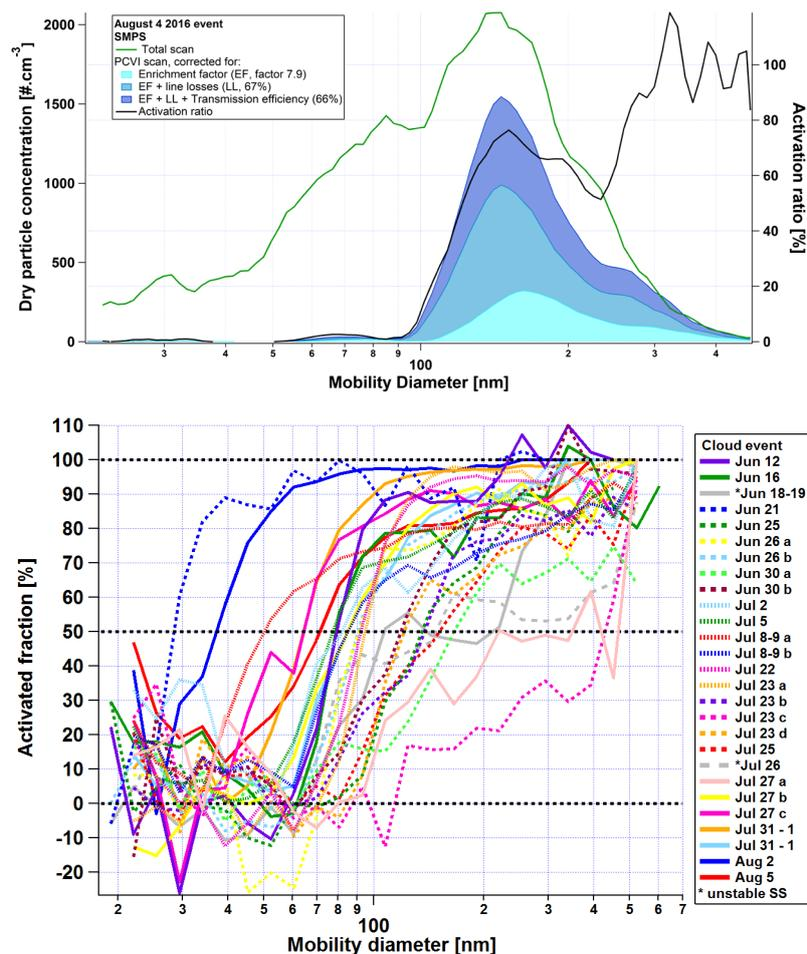
Figure 2. **Top:** Example of the retrieval of the SMPS-derived size-resolved activated fraction using the pumped counterflow virtual impactor (PCVI) and the total inlet, after corrections for lines losses, PCVI transmission efficiency and the enrichment factor. **Bottom:** all SMPS-derived activated fractions using the interstitial and total inlet during the campaign.
