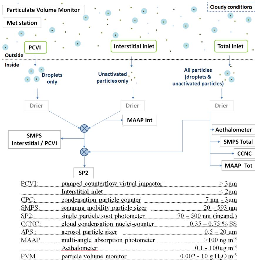
Figure 1. Instrumental set-up during the CLACE 2016 campaign. The total inlet, total SMPS, total MAAP, aethalometer, and the CCNC were part of the Global Atmosphere Watch (GAW) program. “Tot” and “Int” stand for “Total” and “Interstitial”, respectively.
