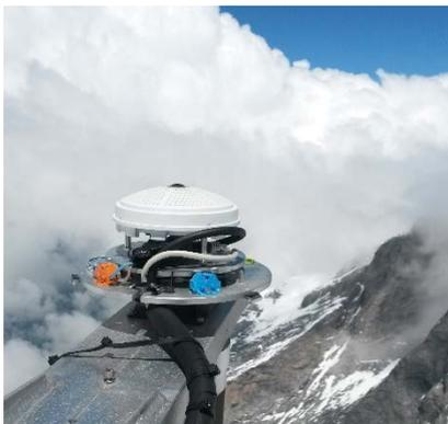
Figure 1. Visible all-sky camera (Mobotix) installed at Jungfrauoch.
