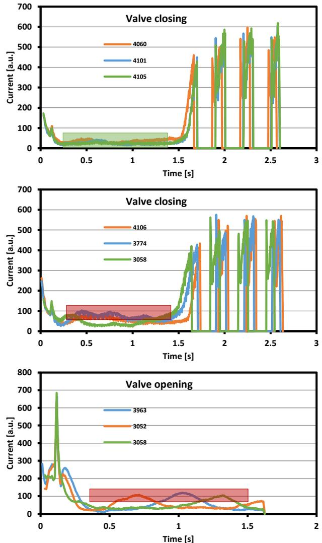
Figure 7. ICOS flask valve current measuring (a) valve closing ok, (b) valve closing bad – current above 72, (c) valve opening bad - current above 72.
