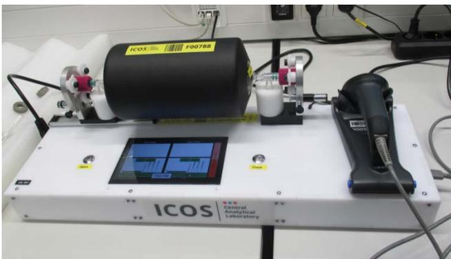
Figure 6. ICOS flask valve test-unit.
