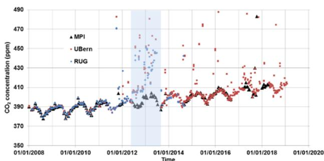
Figure 1. CO<sub>2</sub> concentration as measured by each laboratory. The period from June 12 to August 2013 shaded in light blue corresponds to continuously leaky conditions for the combined UBern and RUG sampling device that progressively increased.
