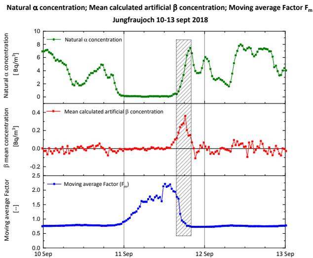
Figure 2. Difficulties of the calculation of artificial betas after period with low alpha concentration on September 11.
