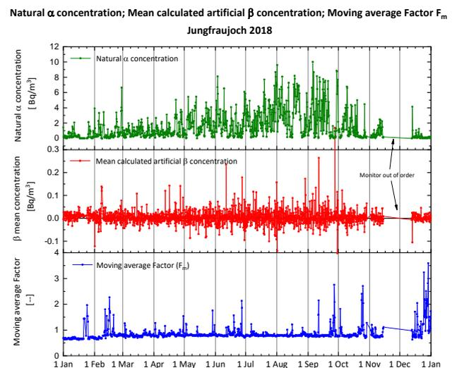
Figure 1. Results of RADAIR measurements in 2018. Top: total (natural)  $\alpha$ -activity concentration; mid: calculated artificial  $\beta$ -activity concentration; bottom: moving average of total  $\alpha$  to total (natural)  $\beta$ -activity. For a better readability, only 4 points per day are represented.
