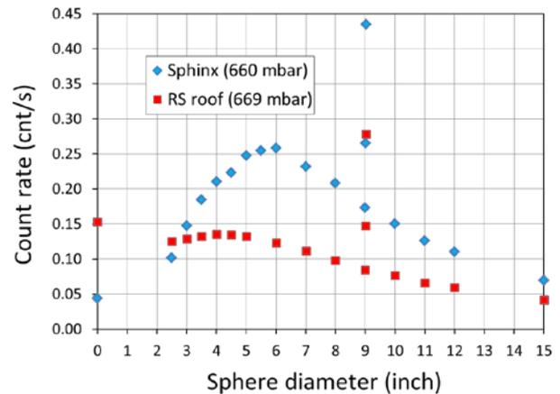
Figure 3. Mean count rates measured by ERBSS in September 2018 in the Sphinx astronomical cupola and below the roof of the RS at Jungfrauoch.
