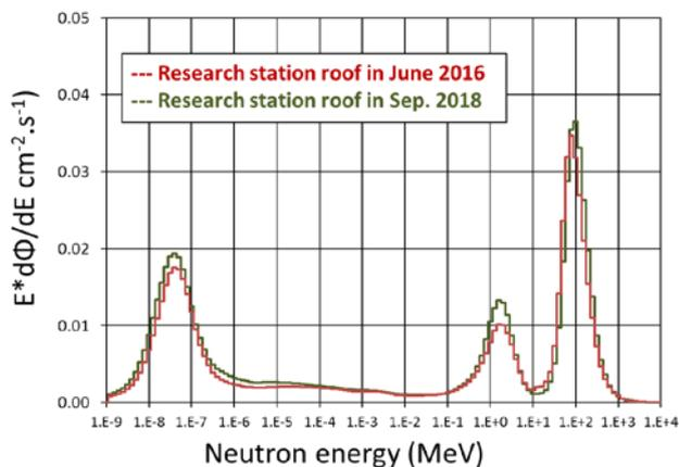
Figure 5. Spectral neutron fluence rate distribution measured in June 2016 and September 2018 below the roof of the research station at Jungfrauoch (corrected to a reference pressure of 669 mbar and solar activity in September 2018).
