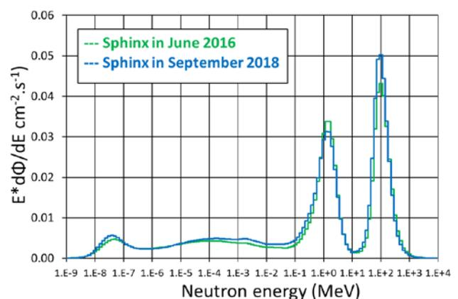
Figure 4. Spectral neutron fluence rate distribution measured in June 2016 and September 2018 in Sphinx astronomical cupola at Jungfrauoch (corrected to a reference pressure of 660 mbar and solar activity in September 2018).
