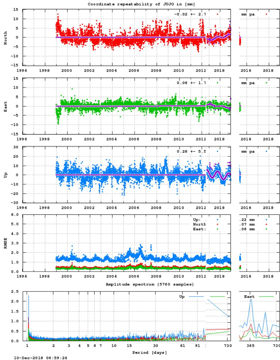
Figure 3. Long-term coordinate estimates for JUJO / JUJ2 (velocities removed; rms and fourier spectrum added).
