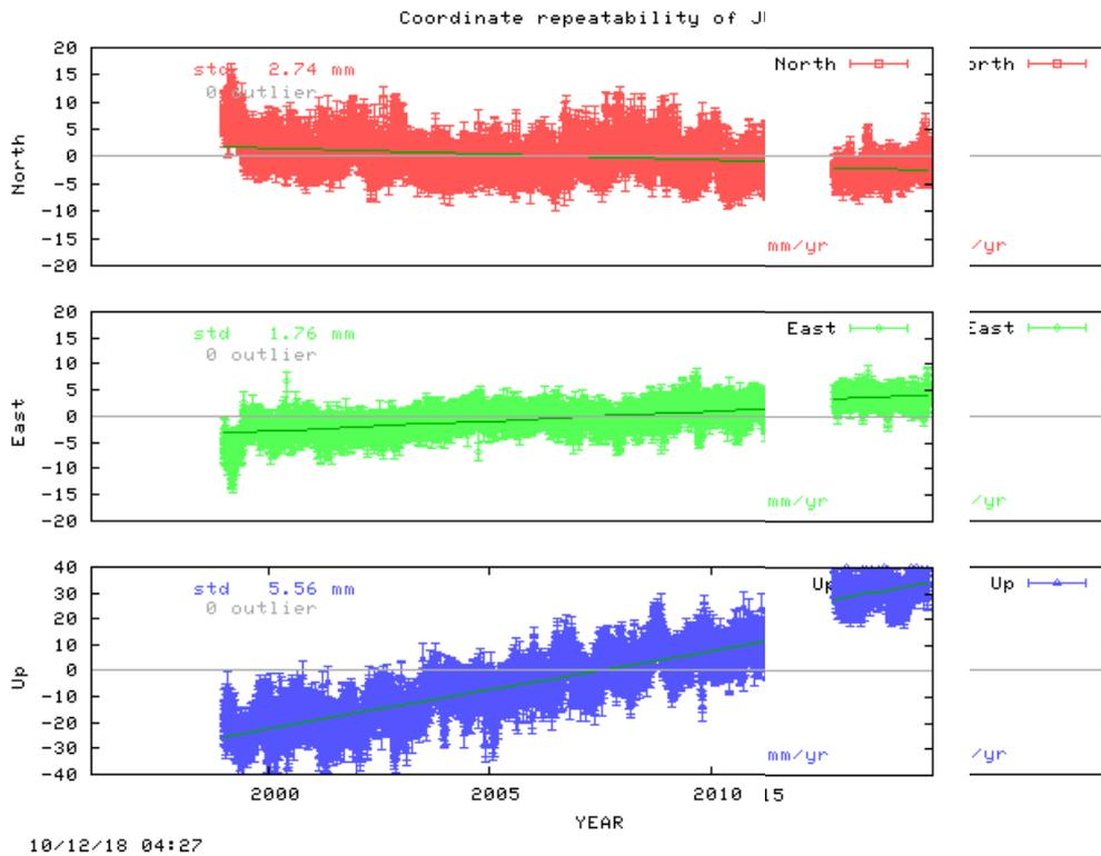
Figure 2. Long-term coordinate estimates for JUJO / JUJ2 (horizontal movement with respect to Zimmerwald, vertical movement w.r.t European Plate).
