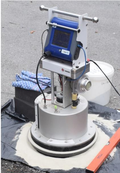
Figure 1. The Portable In-Situ Wind Erosion Lab (PI-SWERL) that can be placed on a surface to determine the PM<sub>10</sub> emitted at a certain friction velocity.
