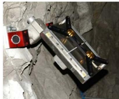
Figure 1. Detector installed and mounted on the bedrock within the Jungfrau railway tunnel. The detector has a view towards the south and is designed to identify the muons that penetrate the interface between the Aletsch glacier and the underlying bedrock (Ariga et al., 2017).
