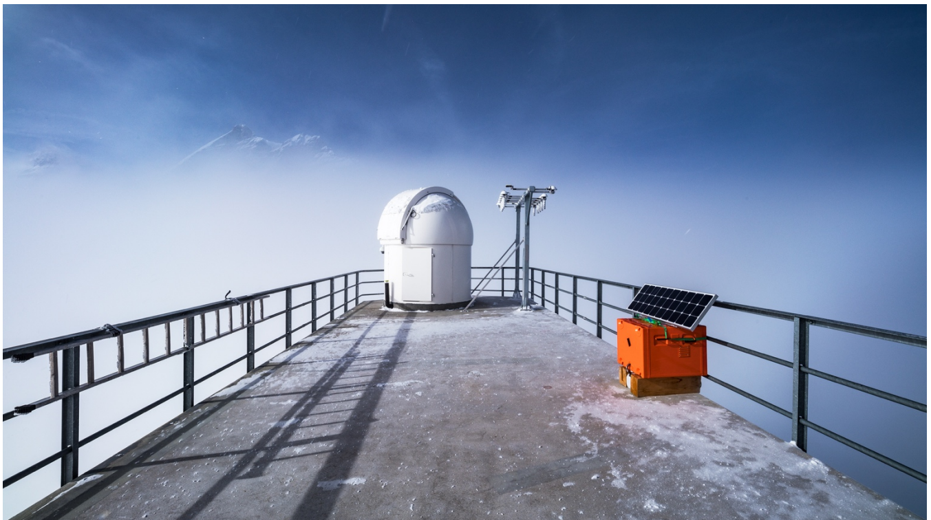
Figure 1. Methanol Fuel Cell in its weatherproof aluminium box with the attached auxiliary solar panel on the lower platform of the Sphinx observatory during the crisp February trials.
