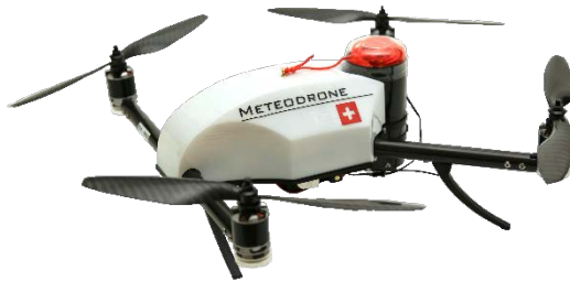
Figure 4. BVLOS certified UAV system Meteodrone.
