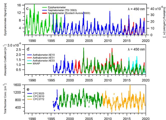
Figure 1 (updated from Bukowiecki et al., 2016). Panels c–e: Temporal evolution of the continuously measured aerosol parameters at the Jungfraujoch (30-day running average of the daily average values).
