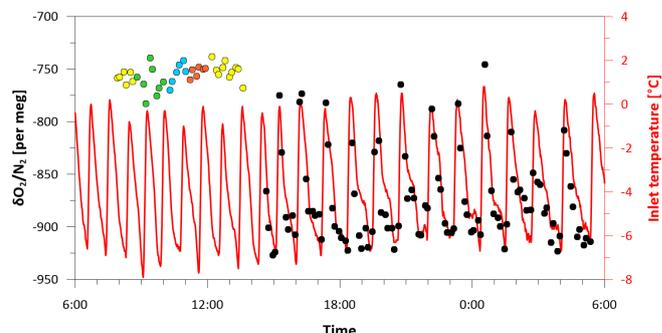
Figure 5.  $\delta O_2/N_2$  values from the first test using a dip tube in the common inlet in different orientations (yellow: opening upwards; green: opening horizontal eastwards; blue: opening downwards; orange: opening horizontal westwards) and without dip tube (black dots), the scale is given on the primary y-axis. The red curve corresponds to the inlet temperature as measured by EMPA with the scale given on the secondary y-axis.
