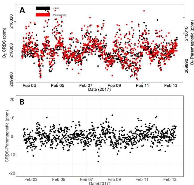
Figure 4. A: O<sub>2</sub> values measured during a 12-day test interval by a newly developed O<sub>2</sub> CRDS from Picarro Inc. and the paramagnetic cell in black and red, respectively, against time. B: Difference (CRDS – paramagnetic) against time. (Berhanu et al., 2019)
