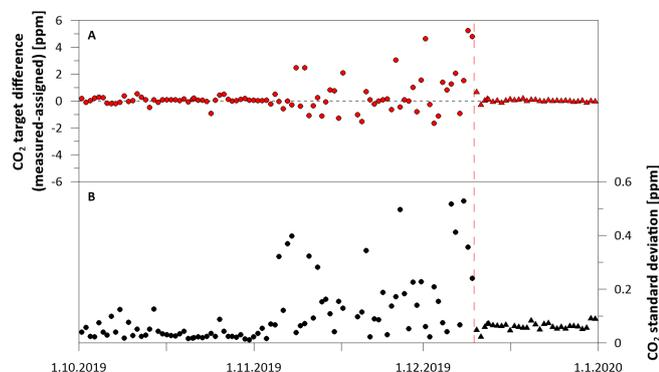
Figure 1. A: Difference of CO<sub>2</sub> target cylinder measurements minus the assigned CO<sub>2</sub> value, red dots represent values before the analyser was replaced (indicated by the red dashed line), red triangles show the same parameter with the new analyser. B: Black
