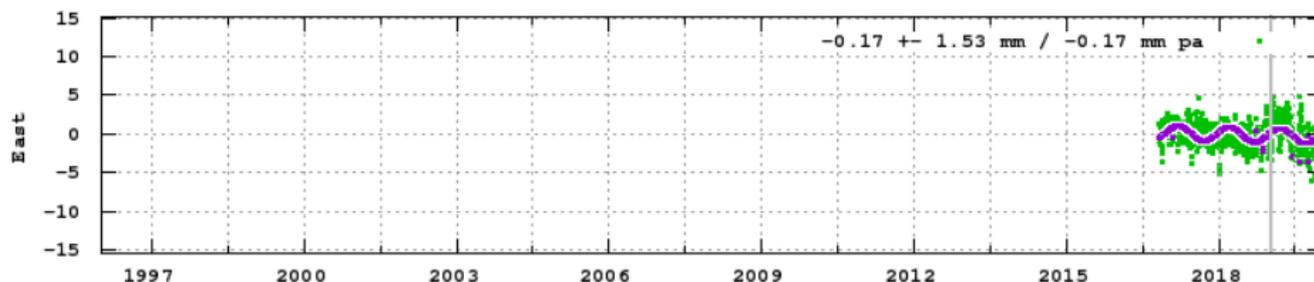
Figure 6. Time series of JUJ2 for the east component in the final coordinate estimation after estimation of an east displacement at Jan. 16, 2019.
