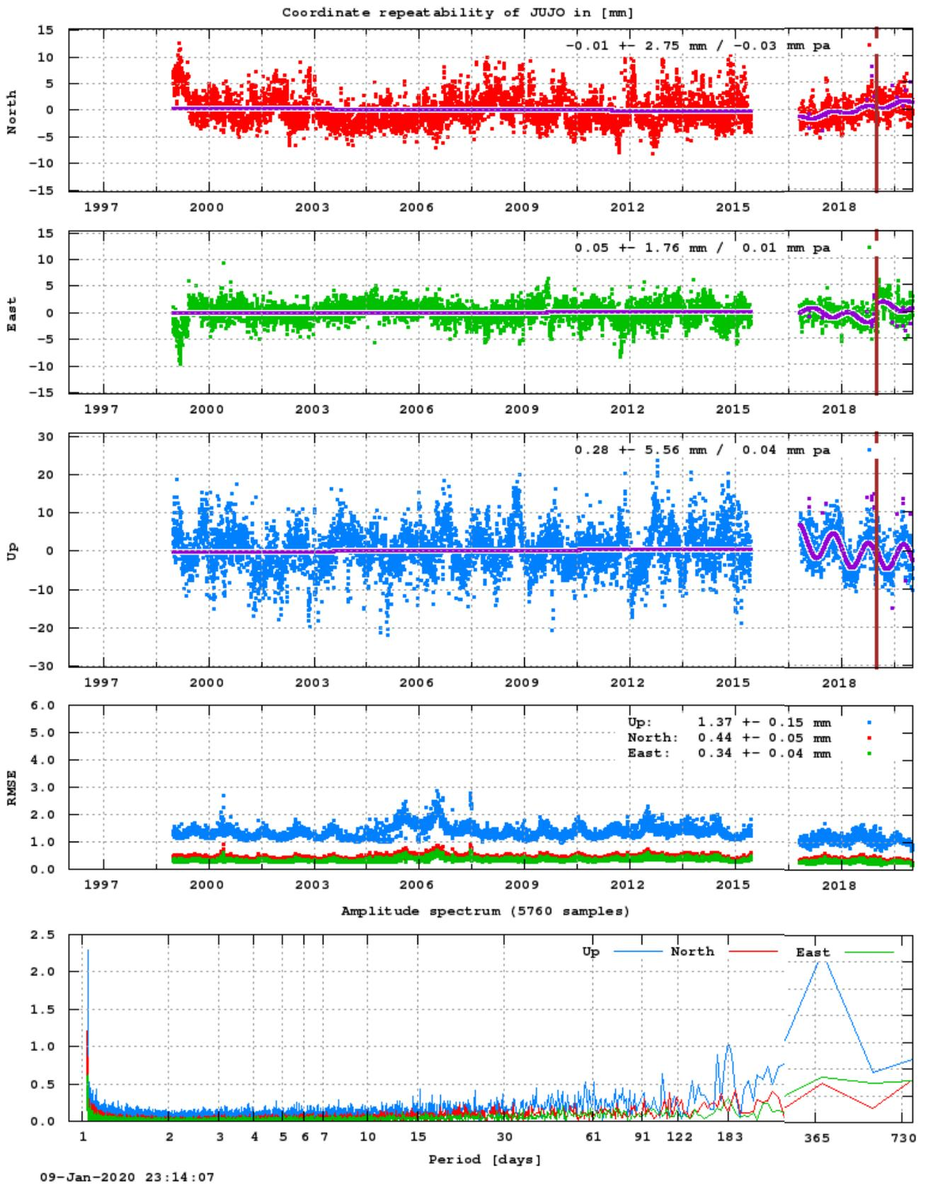
Figure 4. Long-term coordinate estimates for JUJO / JUJ2 (velocities removed; rms and fourier spectrum added; [http://pnac.swisstopo.admin.ch/resplt/juj2\\_fft.gif](http://pnac.swisstopo.admin.ch/resplt/juj2_fft.gif)).
