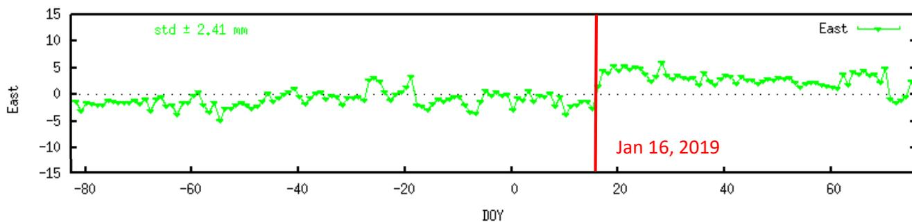
Figure 5. Time series of JUJ2 for the east component in the actual coordinate monitoring when MeteoSwiss removed heavy ice for all sensors of the bridge on Jan. 16, 2019.
