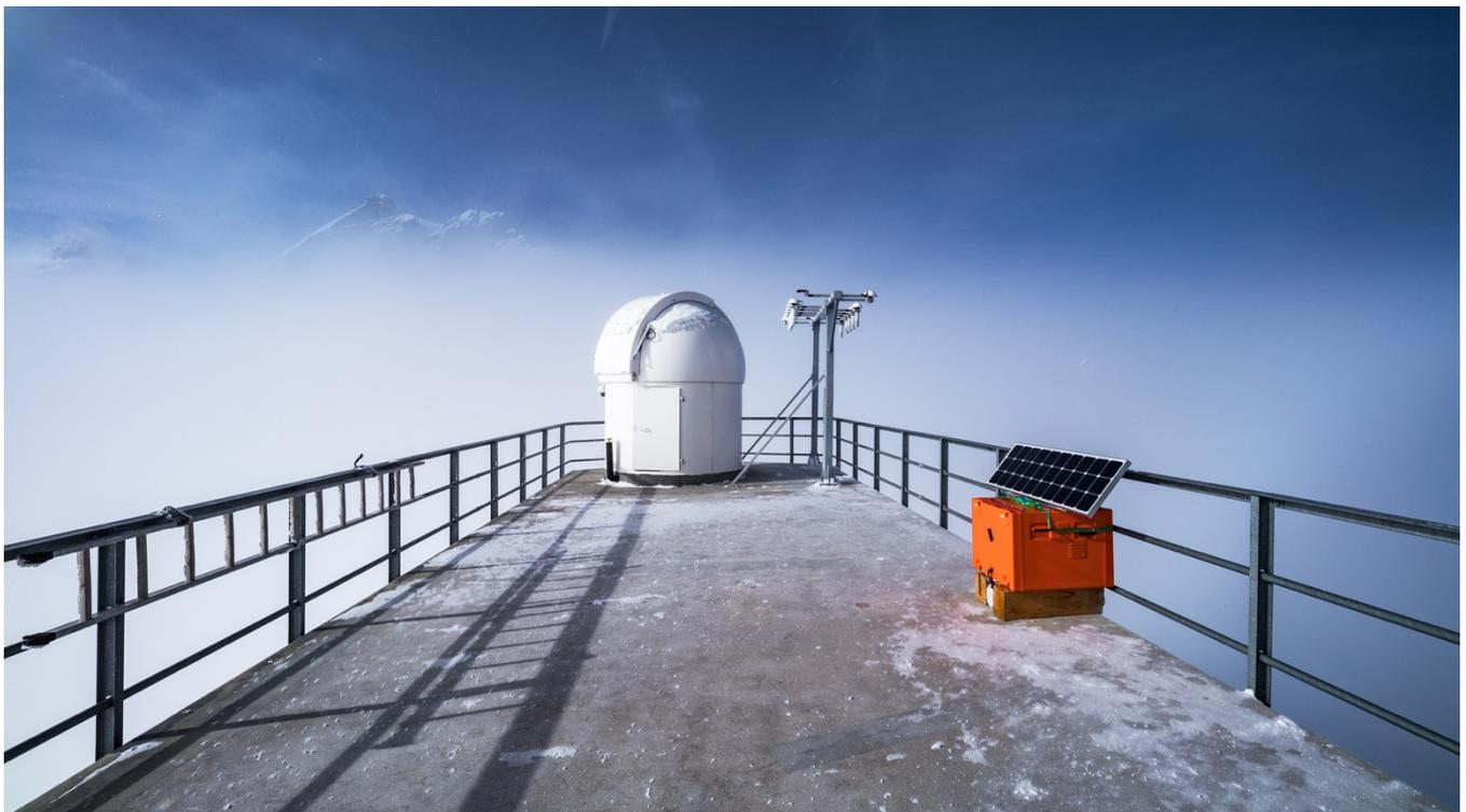
Figure 1. Methanol Fuel Cell in its weatherproof aluminium box with the attached auxiliary solar panel on the lower platform of the Sphinx observatory during the crisp February trials (image from 2018).
