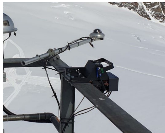
Figure 1. SPN1 pyranometer (on the left in the background) and RoX system, equipped with a moving shadowband (on the right in the foreground).
