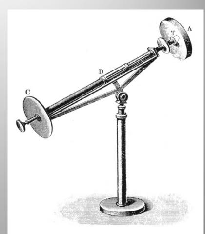
Figure 1. Pouillet's pyrheliometer. A: blackened receiver (metallic container filled with water); T: bulb of thermometer; D, C: alignment check.
